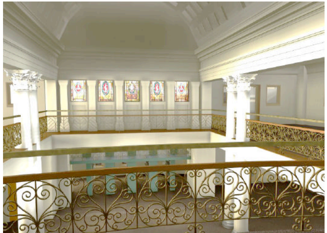
Gallery level with added balcony for exiting. Balcony rail is designed to be compatible but different from historic rail. Although the balcony introduces a new element in the main area of the building, it does not disrupt the overall feel of openness.
